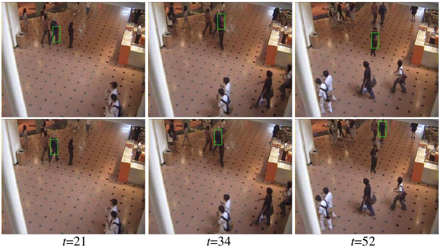
Fig. 3. Tracking results employing RGB as color feature (in the first row) and rgI as color feature (in the second row)
