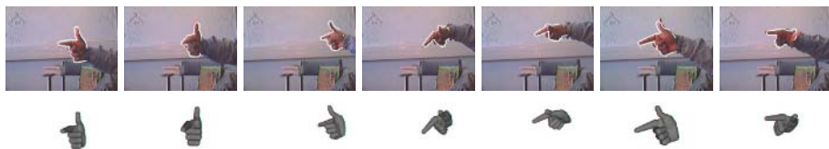
Fig. 5. Tracking a pointing hand. Example frames from tracking a pointing hand sequence with 1100 frames using a single camera are shown. The model contours corresponding to the optimal path through the state distribution are superimposed, and the 3D model is shown below. A total of 389 relevant templates, divided between 10 RVM mapping functions, were used to estimate the hand pose. For comparison, Stenger et al. [18] used 12 000 templates to estimate a similar type of motion.
