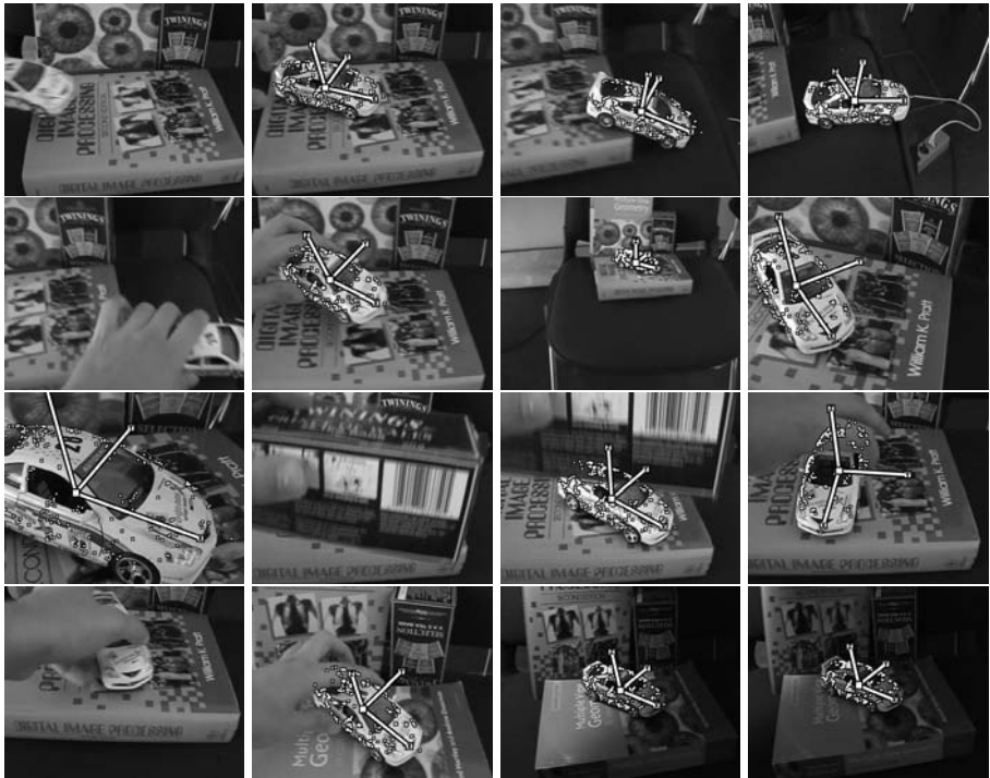
Fig. 5. Detecting the car in a sequence that involves abrupt motions, large scale and lighting changes, and very substantial occlusions. To visualize the results, we attach a 3-D referential to the center of gravity of the initial ellipsoid and use the estimated 3-D pose to project it into the images. We also overlay the projections of the harvested object feature points. The toy car is successfully detected in all frames except those where it is almost entirely occluded. And, because the object is re-detected in every frame, the system easily recovers after such a failure.
