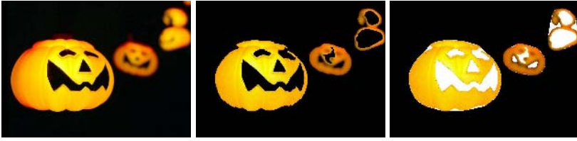
Fig. 6. Demonstrating the shape convexity feature. Left: Original photograph. Middle: Three largest non-background segments shown in original color. Right: Exclusive regions of the convex hull generated for each segment are shown in white. The proportion of white regions determine the convexity value.
