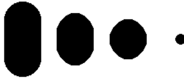
Fig. 5. Euclidean length minimizing flow of a 2D “sausage” (16-neighb). Note that the straight sides have zero curvature and they do not move until the top and the bottom sides (with positive curvature) collapse the “sausage” to a circle.
